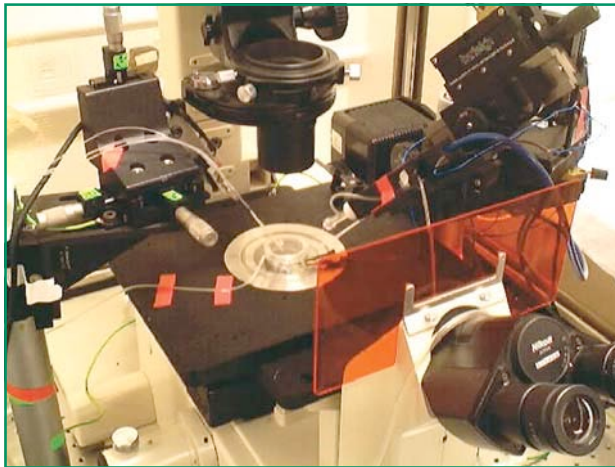
Apparatus used for monitoring the tiny electrical voltages that occur at synapses.
